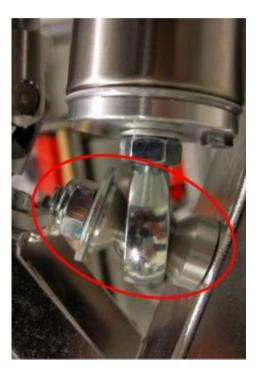
46039 – rotor head III 21,5 • Assemble the upper attachment of the brake / trim cylinder to the rotor head using M6 56/10 A4-80 + 2x spacer and 2x U6 A.
