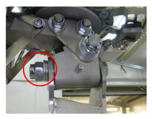
Caution: The forward U13 under the bolt head must not lie on the welding seam!
