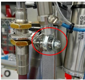
Assemble the roll/trim cylinder to the previously inserted bolt using spacers (angles facing rod end) as shown and secure using U6/18 + M6 Si • Move the rotor head through its full range and ensure there is no blockage of the roll / trim cylinder. If necessary insert a further U6 between PPC roll mounting bracket and inner spacer as shown.
