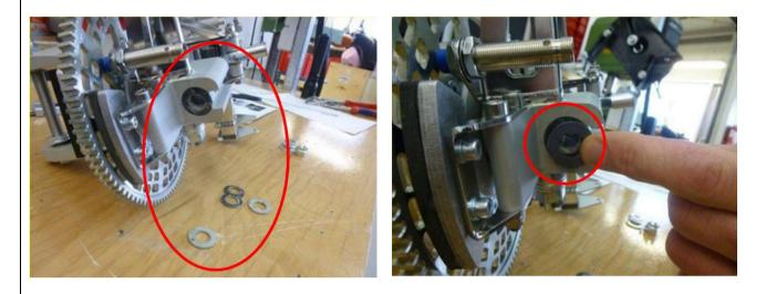
Assemble the rotor head to the mast making sure that all washers are in place and secure using the gimbal bolt + U13. Fit the castle nut M12 and 2x washer U13 as shown.
