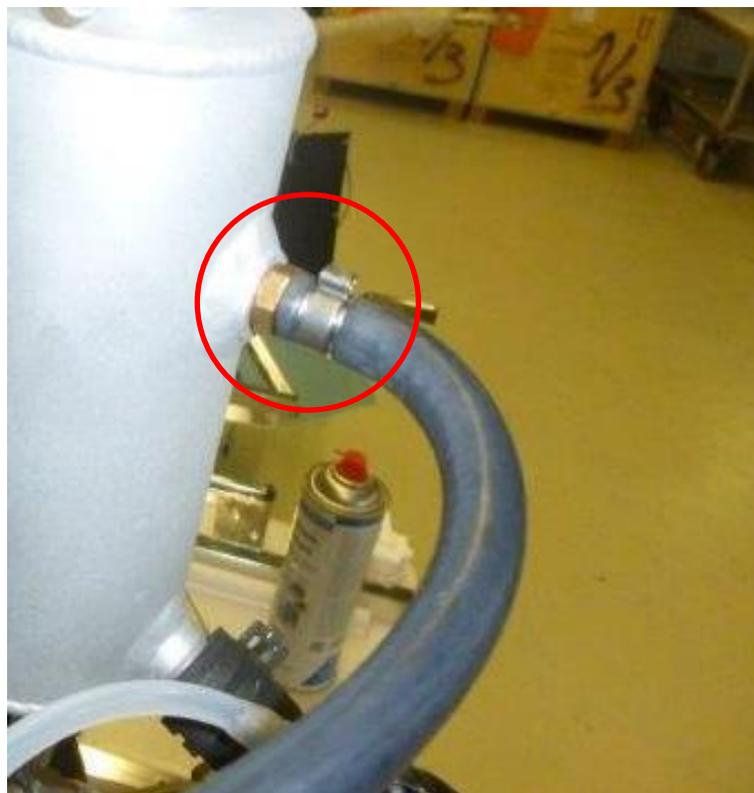
Fig.4: Nipple with copper washer and crimp
