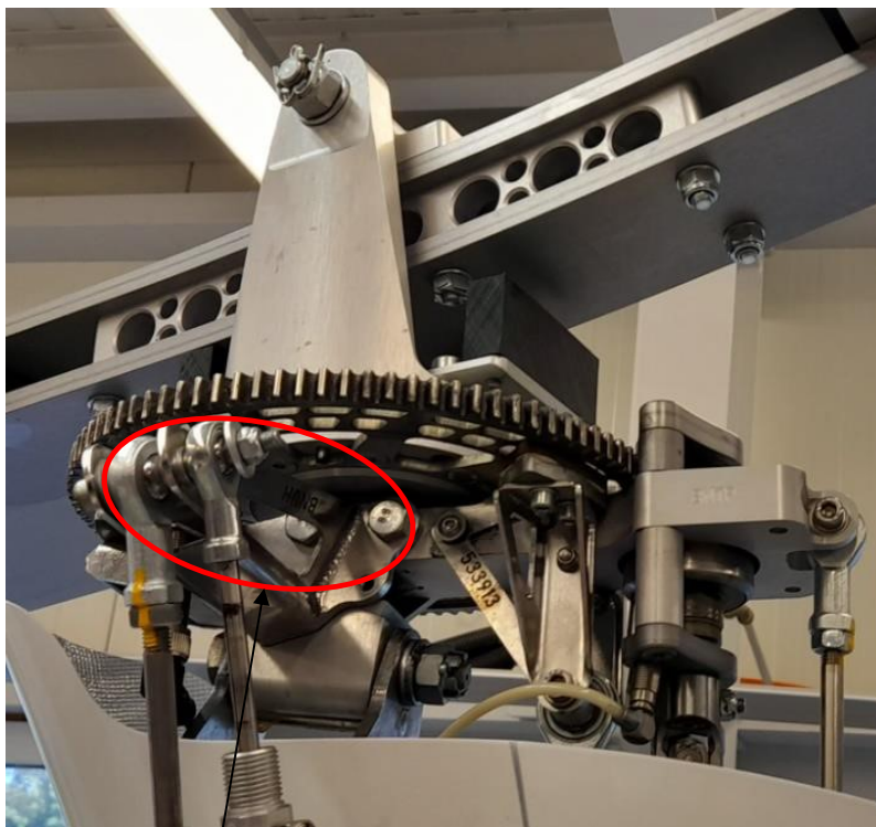
The ringed area indicates the installed bridge linkage
