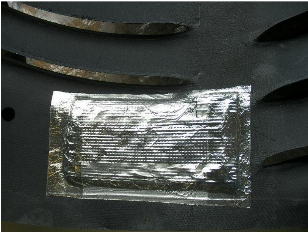
Fig. 2 - Mounted Heat Protection Engine Cowling
