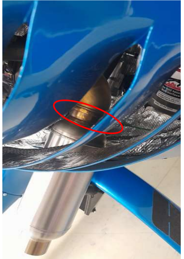
Welding seam is visible with installed cowlings
