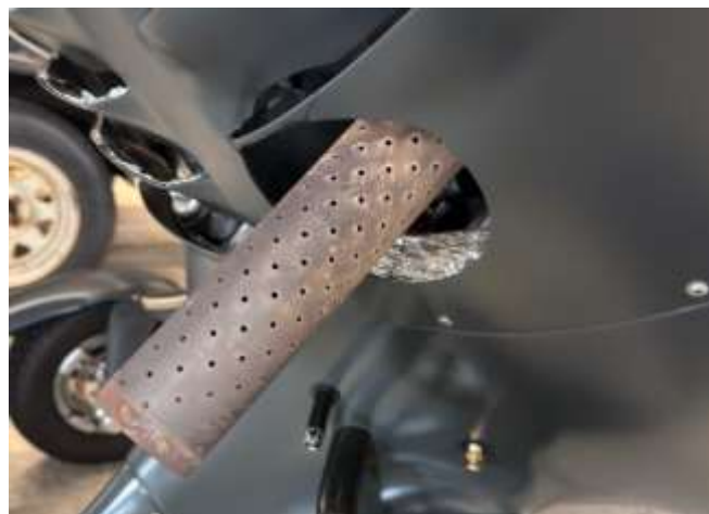
Remains after the aftermuffler shell has detached in flight
